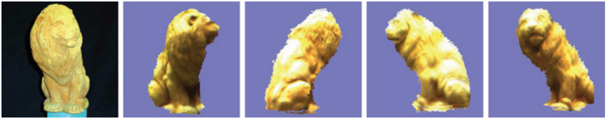
Figure 12: RGBz light field example from [TRSKK08], where a PMD Vision 19k cameras was used. The artefacts result from the inaccurate depth information at the object boundaries.
