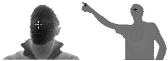
Figure 10: Left: Sample nose-detection results shown on ToF range image; detection error rate is 0.03 [BHMB08b]. Right: The direction the user is pointing in can be computed from the difference vector between the positions of the head and hand [HBMB09].
