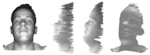
Figure 4: Improvement of range map quality using the shading constraint. From left: Intensity image; lateral view of raw measured surface and surface reconstructed using the shading constraint in lateral and frontal views.
